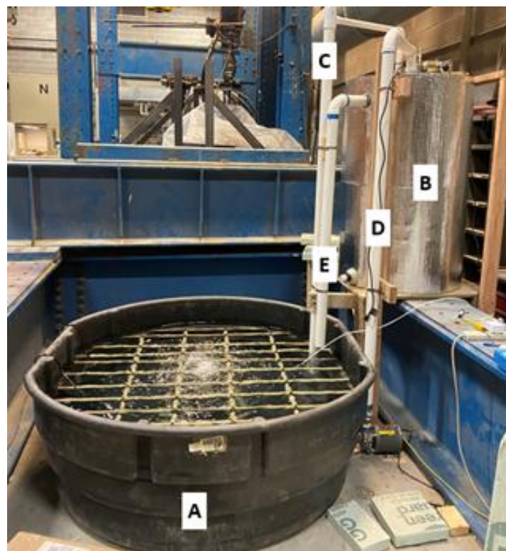
Figure 2: Accelerated corrosion setup depicting A) exposure tank, B) reservoir, C-E) piping.
