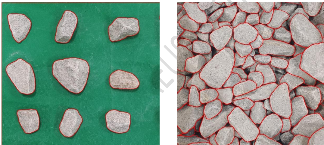
Figure 2: Schematic illustration of particle contour extraction through image segmentation: segmentation of particles in dispersed state (left) and segmentation of particles in densely packed state (right).
