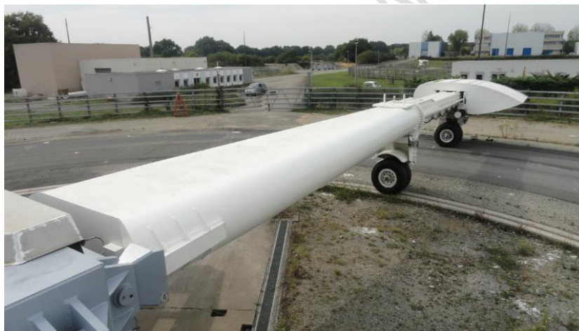
Figure 1: Photo of one of the four arms of the Université Gustave Eiffel's accelerated pavement testing facility: Fatigue carousel.
