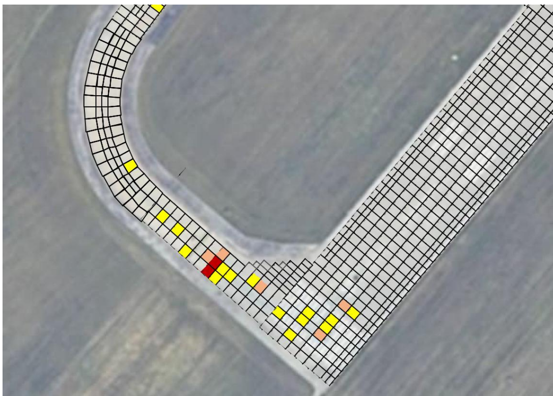
Figure 1: Broken slab corner defect occurrence map.
